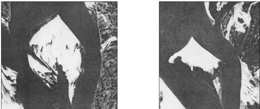
Figure 3.19: Two examples of braid bars in the Jamuna River from which flow direction can be derived (in both cases from top to bottom).
